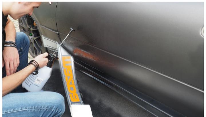
Once the front of the sticker is glued, the same procedure is reproduced on the back of the sticker in increments of 60 to 80 cm.
