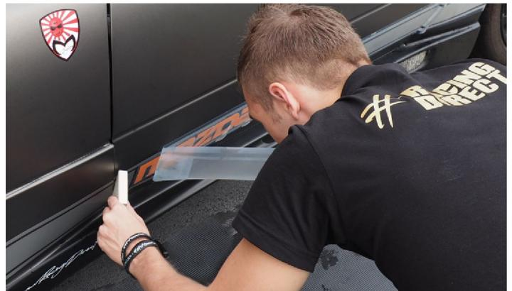
Remove the transfer film **very gently**. The sticker must remain glued to the body.
