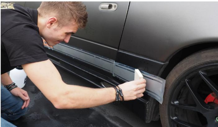
Thoroughly press to remove water and air bubbles.
